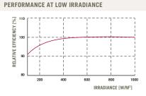
Typical module performance under low irradiance conditions in comparison to STC conditions ( $25\,^{\circ}$ C, 1000 W/m<sup>2</sup>).
